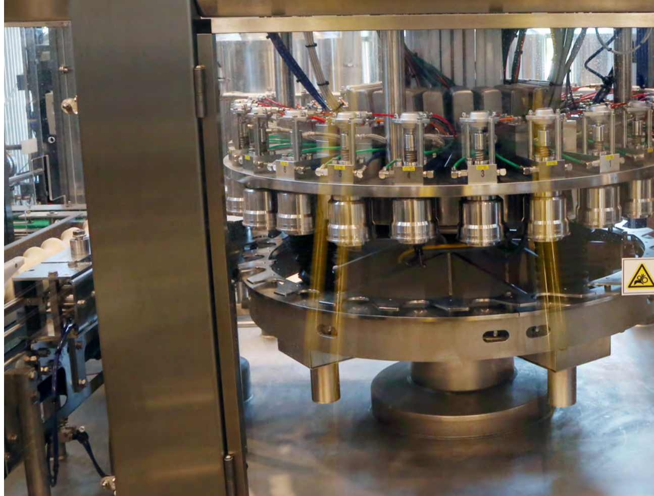
Capable of reaching throughput speeds of up to 240 cans per minute, the Krones Craftmate canning line at Cowbell Brewing comprises a rotary 24-head volumetric filler and a Krones Checkmat inspection system ( inset ) using X-Ray inspection to ensure accurate and consistent fill levels in each can of beer coming off the canning line prior to case-packing.
