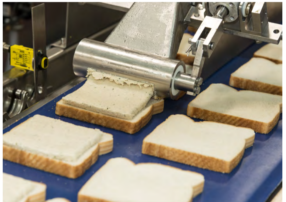
A close-up view of a Reiser Vemag spreading a meat filling on the bottom slice of a bread sandwich on one of Aliments Martel's four production lines.
