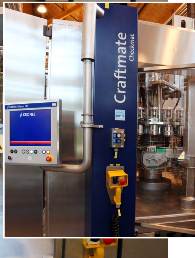
Capable of reaching throughput speeds of up to 240 cans per minute, the Krones Craftmate canning line at Cowbell Brewing comprises a rotary 24-head volumetric filler and a Krones Checkmat inspection system ( inset ) using X-Ray inspection to ensure accurate and consistent fill levels in each can of beer coming off the canning line prior to case-packing.
