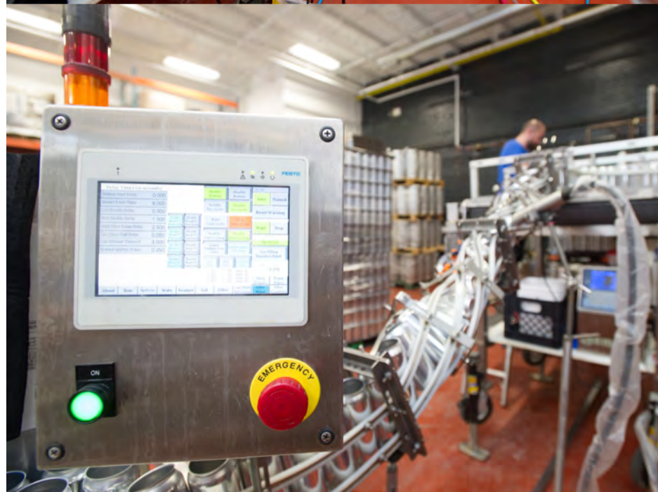
After the Ball Corp. manufactured aluminum cans brought to the brewery by Sessions Craft Canning flipped upside down and cleaned, an EBS 6500 coder applies lotcode and best-before data to each individual container.
