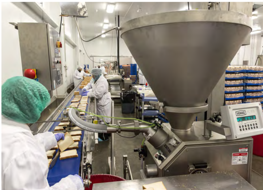
Avoiding excess product layers by human hands, a Reiser Vemag applies a controlled, even layer of meat spread onto a slice of sandwich bread at the Aliments Martel facility.
