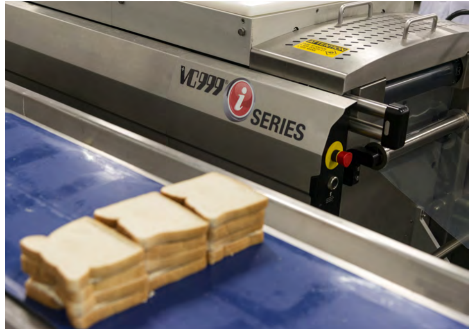
Close-up of sandwiches on a conveyor line, awaiting primary packing via a VC999 i-Series 423 thermoformer with Videojet inkjet printer.
