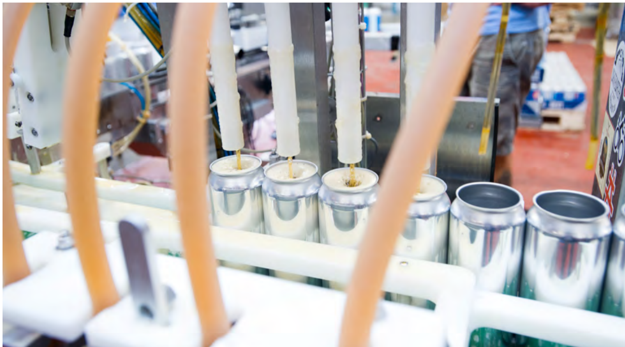
A close-up of one of the Wild Goose canning lines filling four cans at a time used by Sessions Craft Canning in its traveling filling-line business.
