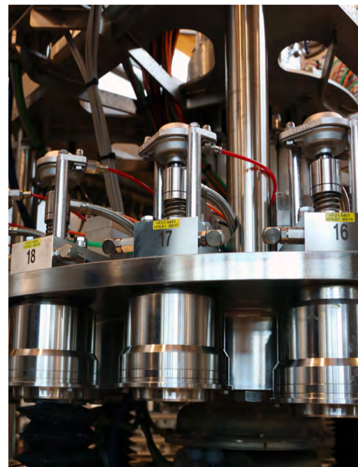
A close-up of the high-precision filling valves inside the Krones Craftmate rotary filler integrated with a four-head Ferrus seamer in highly efficient configuration to ensure low oxygen content in the canned beer products.
