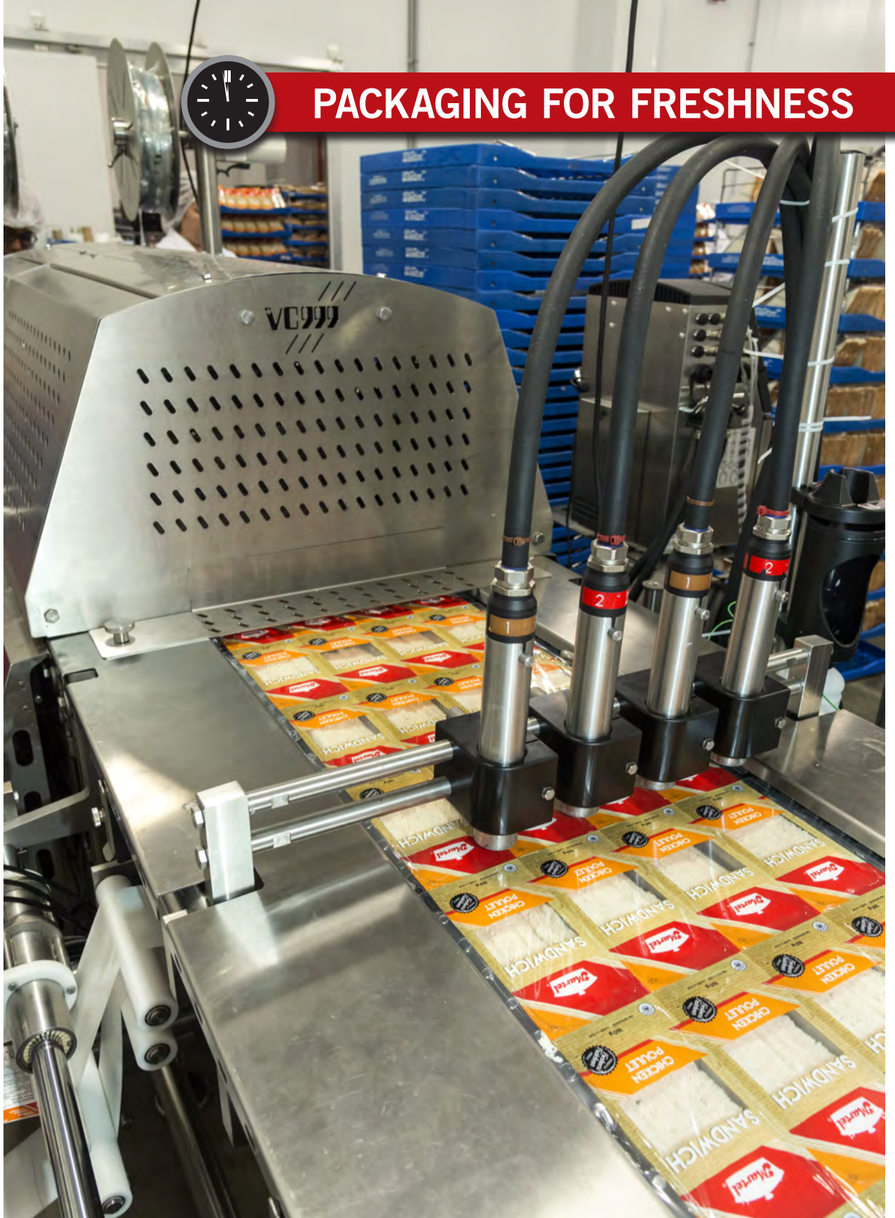
A Videojet inkjet printer mounted to a VC999 i-Series 423 thermoformer applies best-before and lot code data to individual sandwich backs at the Aliments Martel facility in Terrabonne, Que.
