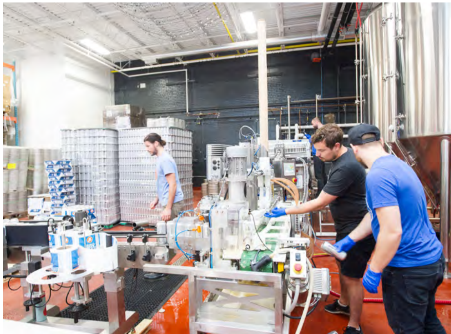
Sessions Craft Canning travels to Toronto, Ontario Henderson Brewery with two workers and a portable canning line to fill, seal and label its beers at a rate of about 900 liters per hour.
