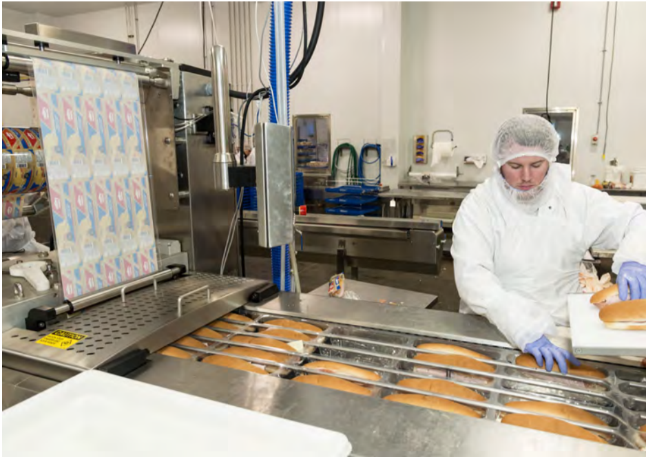
An Aliments Martel employee hand-places sub sandwiches onto the lower pocket of film before being sealed by a VC999 i-Series 459 thermoformer.
