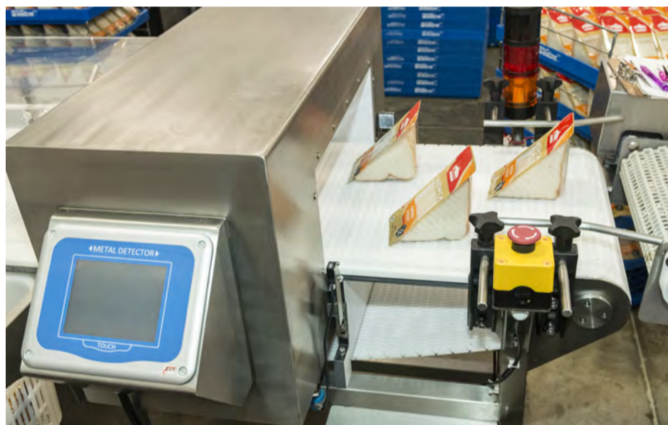
A VC999 XtraVac Metal Detector 4121 unit inspecting individual sandwich packs sealed by a VC999 thermoformer.
