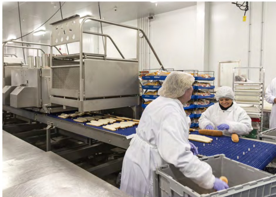
Aliments Martel employees place bread onto a conveyor that moves under a Grote slicing machine that deposits slices of meat onto the open-face sub bread.
