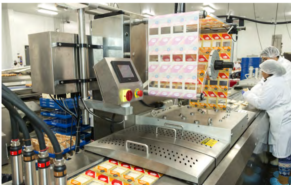
Workers place two halves of a sandwich into each lower film pocket before a VC999 i-Series 423 thermoformer applies a top layer of film to seal it. An attached Videojet inkjet printer then applies lotcode information and best-before date onto each pack of chicken sandwich.
