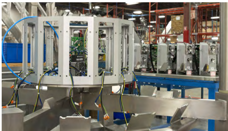
A close-up of a workstation used to assemble the PrimoCombi range of multihead weighing systems for high-performance applications requiring high throughput rates and tight accuracy tolerances in busy or harsh production environments.
