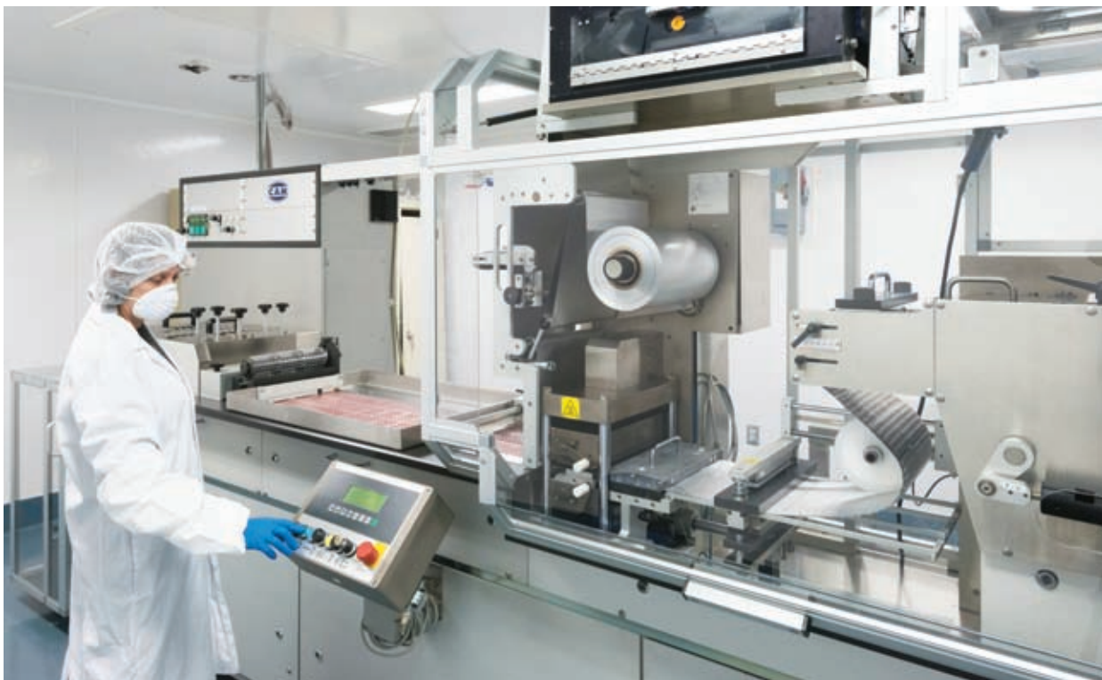
Machine operator making on-the-fly adjustments to the blister-packing machine boasting inline printing capabilities.
