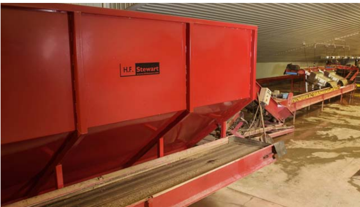
Along with an Even Flow Hopper and Steel Drum washer, Monaghan Farms uses a felt drier for processing of its harvested potatoes, with P.E.I.-based H.F. Stewart supplying all of this equipment.
