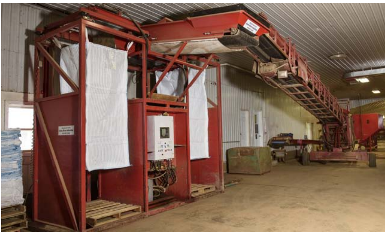
Monaghan Farms uses an automatic tote filler from Dunk River Industries to fill 3,400 pound bags in under two minutes, with an elevator lifting empty bags up to the top, and lowering them slowly as it fills to prevent product damage.
