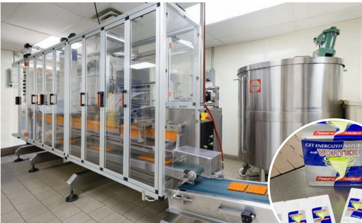
A high-speed, fully-automatic form/fill/seal machine used to produce the popular double-sachet packs (inset) widely used for sample packs and promotional giveaways.
