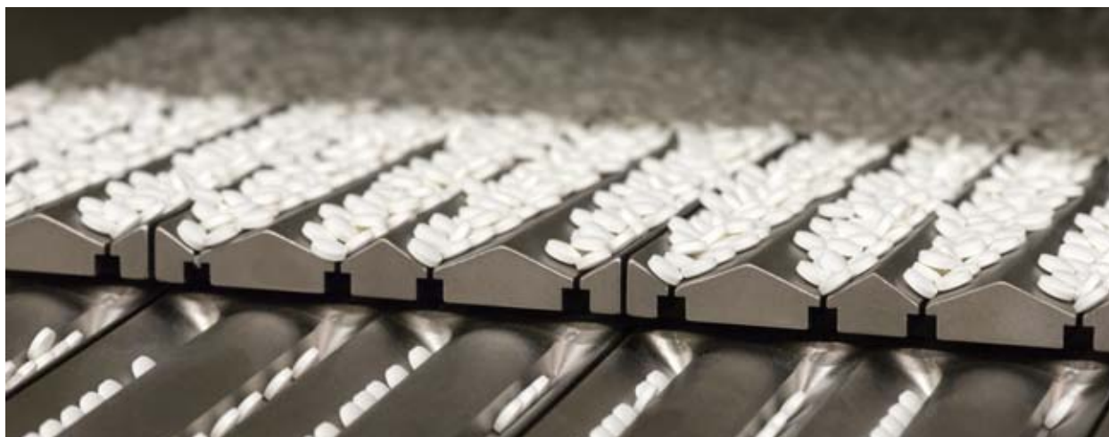
A close-up of— tablets being counted and aligned for filling inside the Street Fighter SF-100 electronic tablet counting machine from Capmatic, which can handle a broad range of pill types and work with a variety of different container sizes and shapes at maximum throughput speeds of up to 120 bottles per minute.
