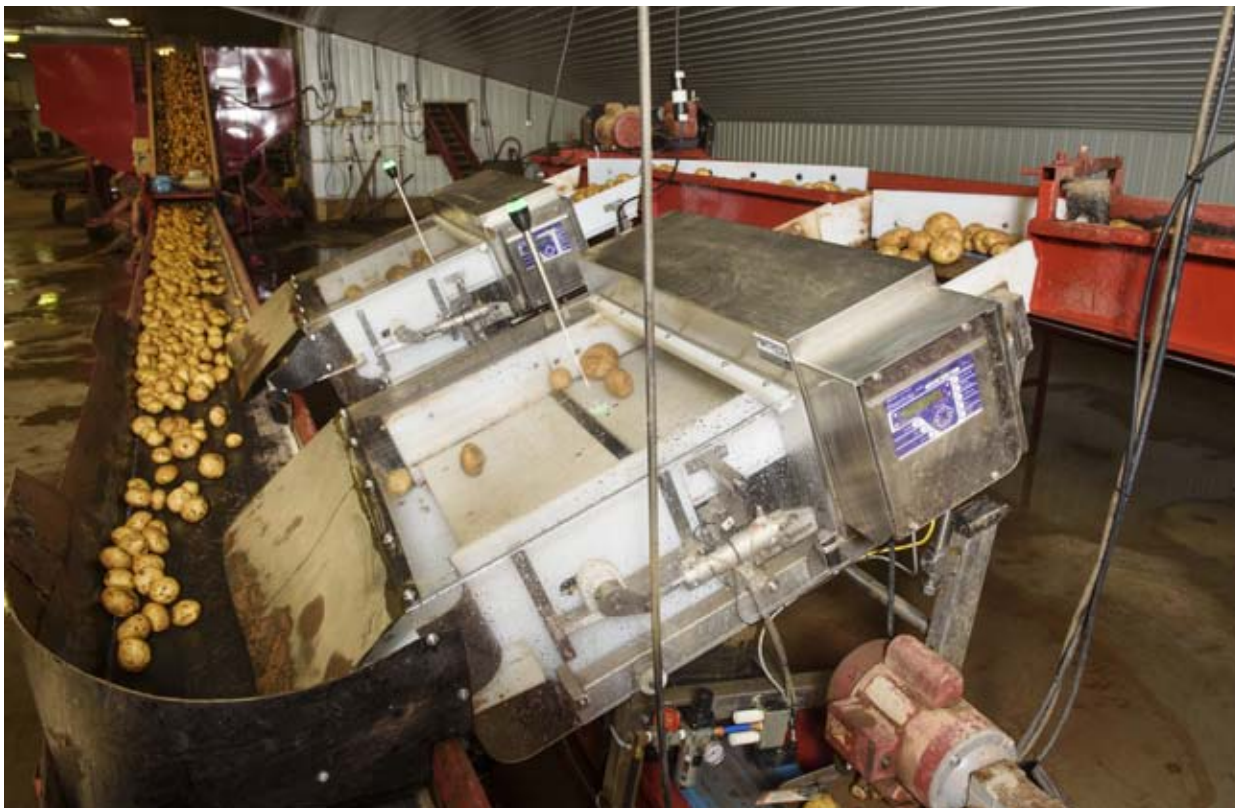
To ensure optimal levels of food safety for consumers and customers, Monaghan Farms added three special Phantom metal detection systems from Fortress Technology to inspect all of its raw products.
