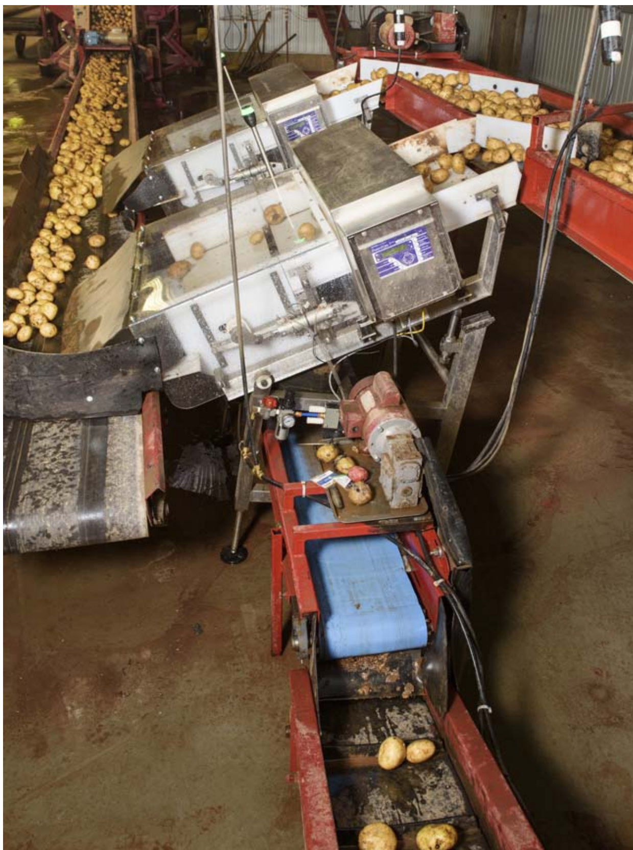
Two Bulk Potato Retract metal detection systems used by Monaghan Farms at its Prince Edward Island facility, are specially-designed from a basic Phantom metal detection unit specifically for the potato processing market segment.
