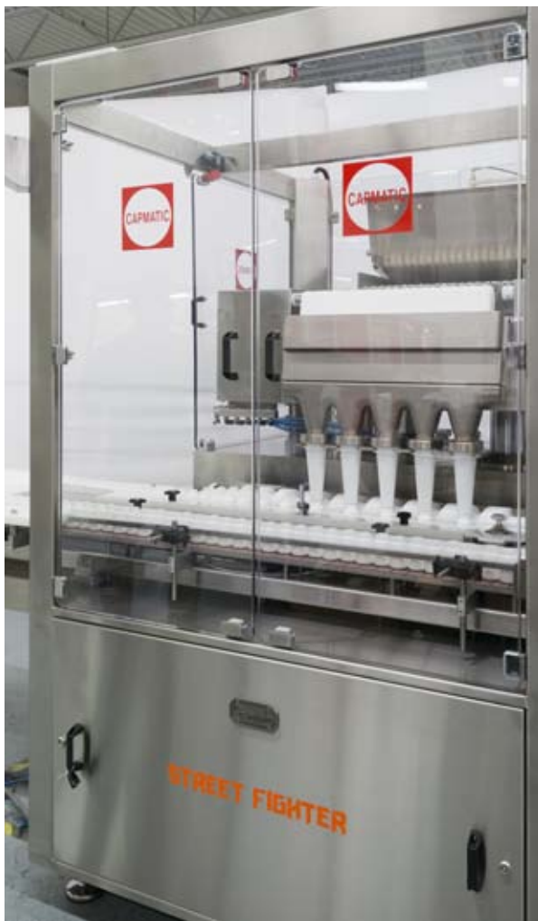
The Street Fighter tablet counter can achieve throughput speeds of 100 bottles per minute for 100-tablet bottles.
