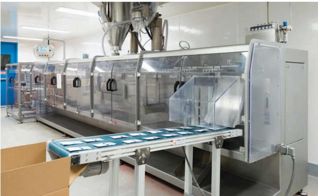
Packages coming out of the high-speed form/fill/seal unit-dose packaging machine are conveyed into the shipping box.
